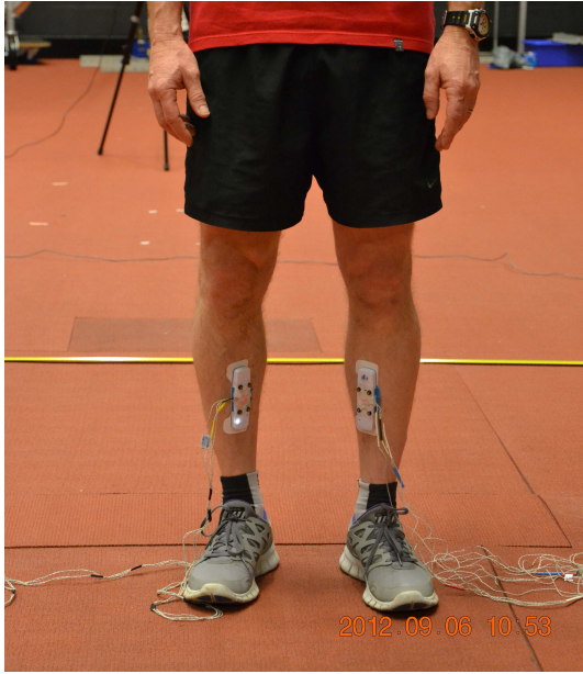
Fig. 1. Subject wearing two ViPerform sensors on the tibia.
