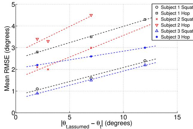
Fig. 5. Mean RMSE values of tibia-adduction angle with respect to the difference between  $\theta_t$  and its assumed value  $\theta_{t,assumed}$ .
