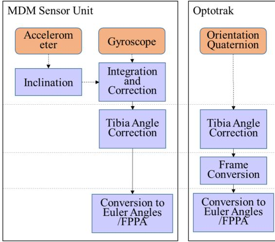
Fig. 2. Processing Flow for Sensor and Optotrak Data.
