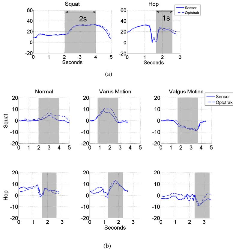
Fig. 3. Example (a) tibia-flexion angle and (b) tibia-adduction angle from squat and hop tests, compared with Optotrak. Grey area shows the period of motion.
