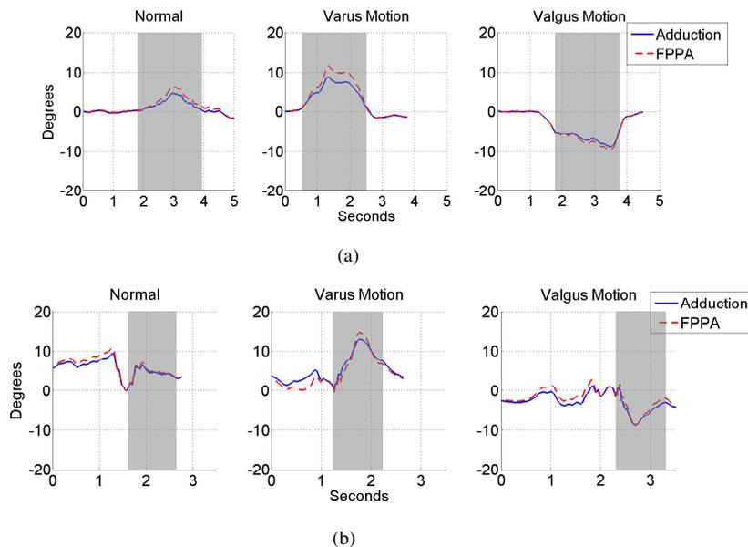
Fig. 4. Comparison between tibia-adduction angle and FPPA in example (a) squat and (b) hop tests.
