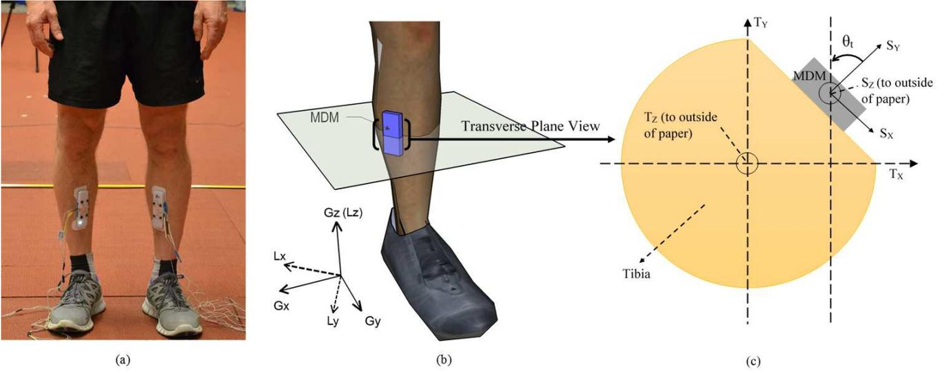
Fig. 1. Sensor placement from different view. (a) Two sensor units placed on left and right tibia of subject 1 (coronal plane view). (b) Sensor unit placed on left leg, showing lab-CS and global-CS. (c) Transversal plane view of sensor placement on the left leg, showing sensor-CS, tibia-CS and the angle  $\theta_t$ .
